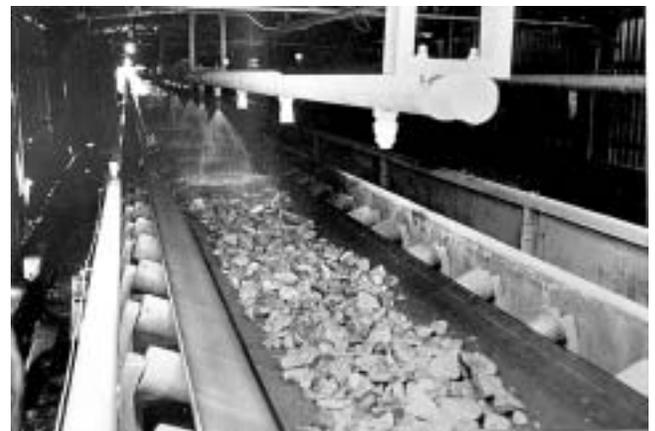
Fig. 4.5—Cooling coarse aggregate by chilled water spray and inundation.
