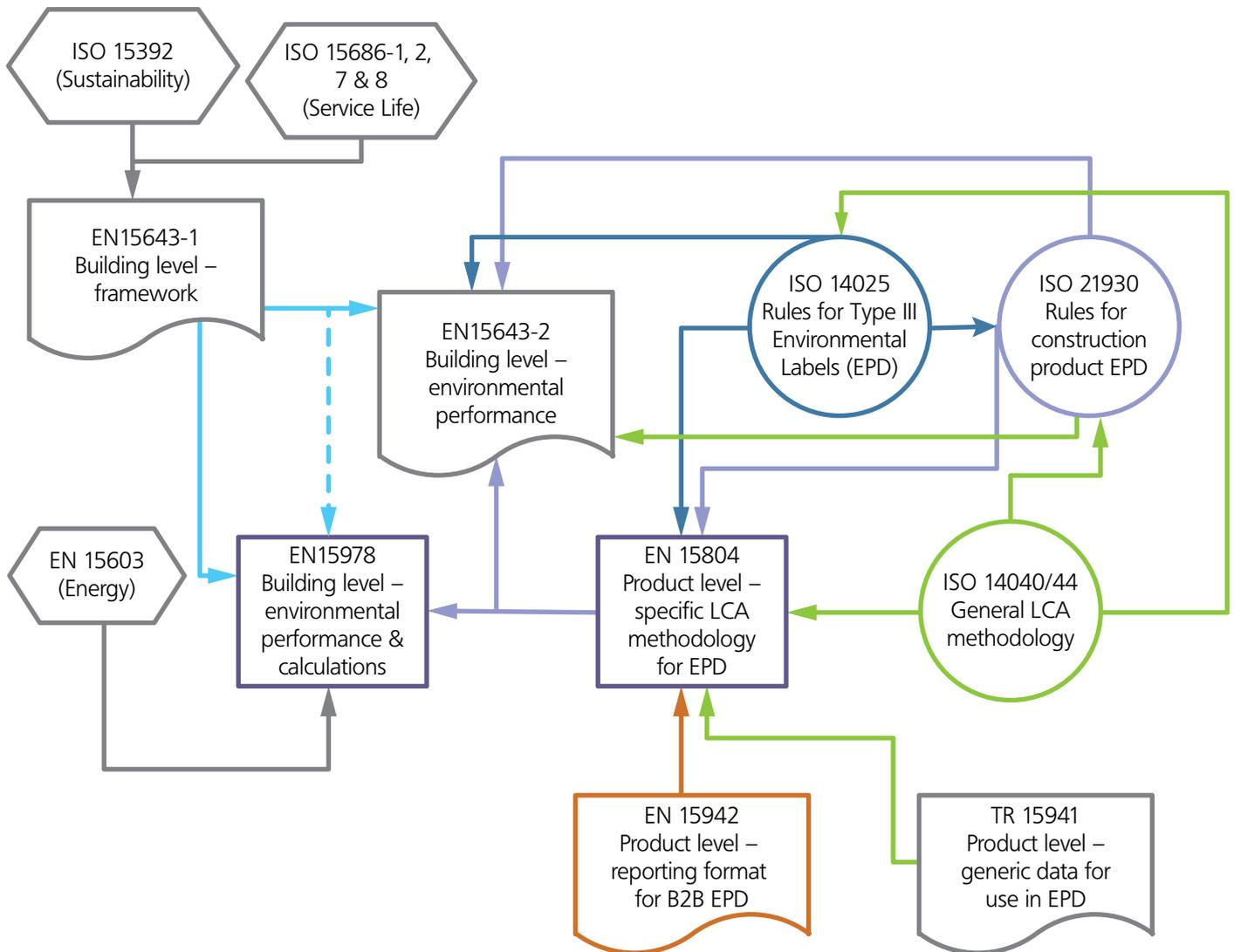
**Figure 2: Interactions between TC 350 environmental assessment EN and ISO standards**
