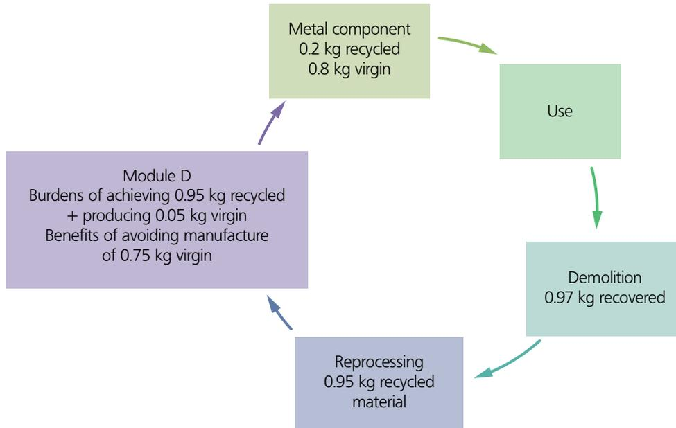
**Figure 4: Diagram of example Module D scenario**
