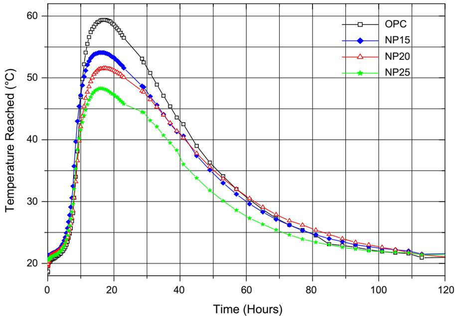
Figure 8. Temperature reached by mortar versus time.
