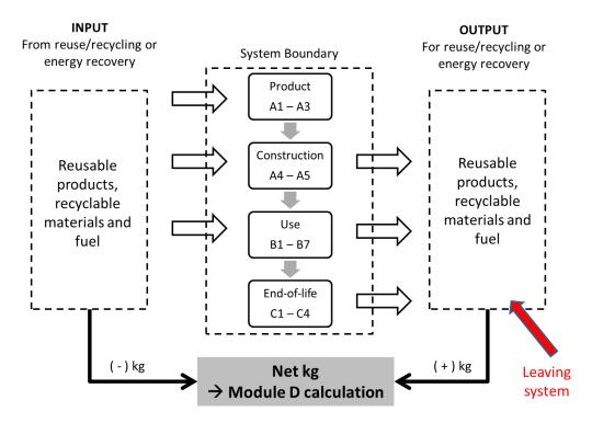
Figure 6.1: Module D Principles
