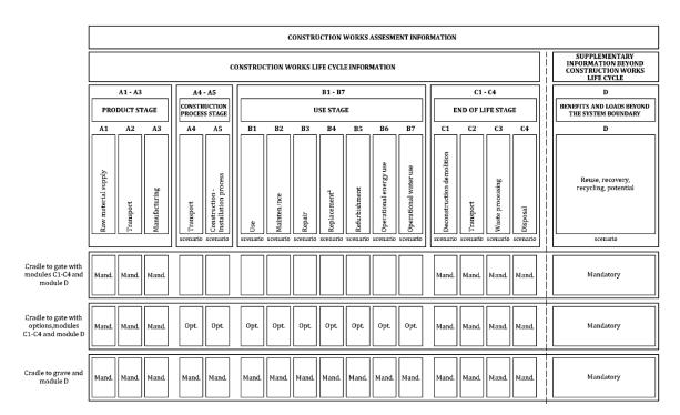
Figure 5.1: Illustration of mandatory and optional elements and information modules for construction products, adapted from EN 15804+A2
