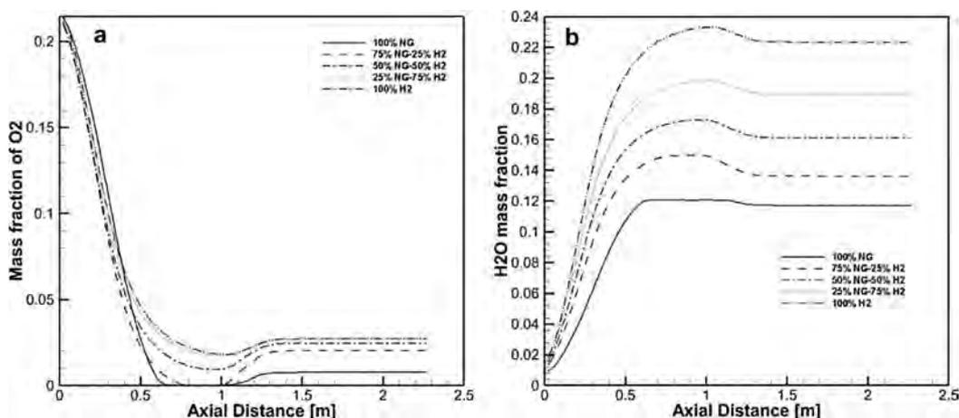
Fig. 11 – The comparison of the natural gas and hydrogen-enriched natural gas a) axial O<sub>2</sub> distribution at the center line, b) axial H<sub>2</sub>O distribution.
