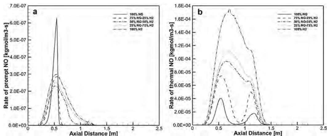
**Fig. 7 – The comparison of the natural gas and hydrogen-enriched natural gas a) axial rate of prompt NO distribution, b) axial rate of thermal NO distribution at the center line.**
