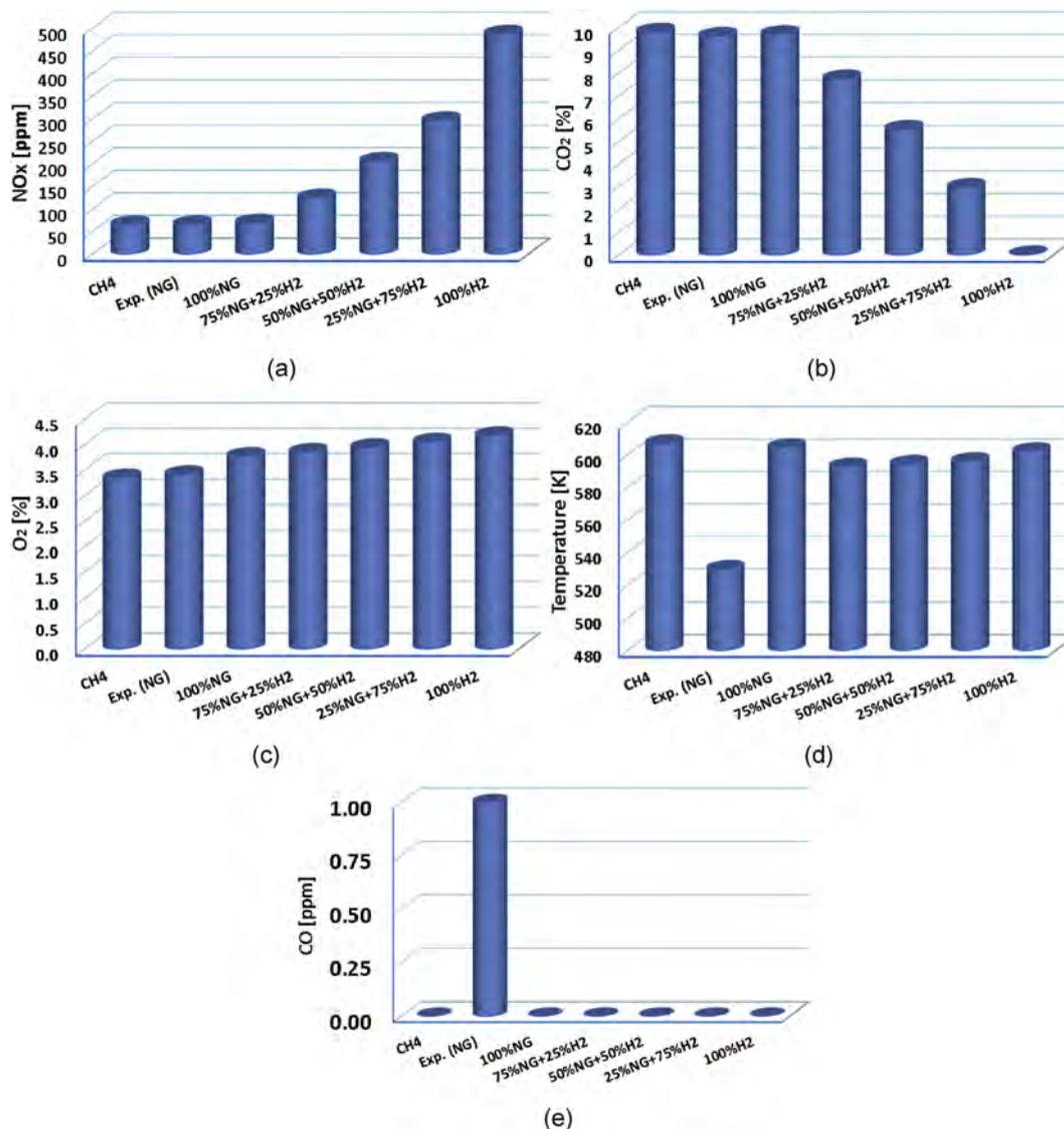
**Fig. 12** – The comparison of the combustion products and outlet temperature ( $T_{out}$ ) of studied fuels a) NO<sub>x</sub> emissions, (b) CO<sub>2</sub> emissions (c) O<sub>2</sub> species (d)  $T_{out}$  measurement (e) CO emissions at the boiler outlet (stack inlet).
