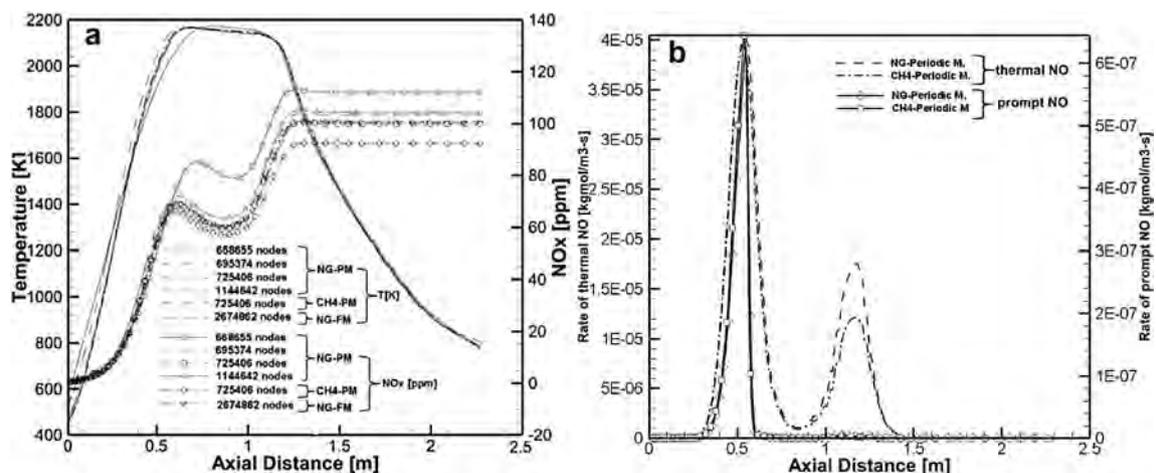
**Fig. 4 – Comparison of geometric models and fuel characteristics of natural gas and methane considered the temperature distribution and NOx gradients a) axial temperature and NOx gradients for different nodes number b) axial rate of thermal NO and rate of prompt NO on yz plane.**
