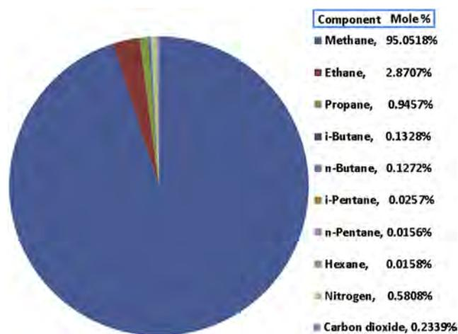
Fig. 2 – Components of natural gas [26] used in testing and numerical simulations.
