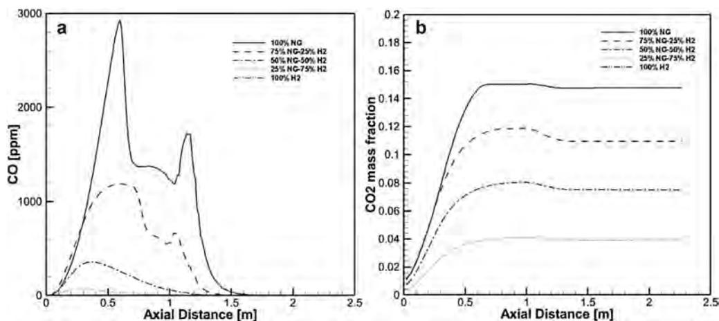
Fig. 10 – The comparison of the natural gas and hydrogen-enriched natural gas a) axial CO distribution, b) CO<sub>2</sub> distribution at the center line.
