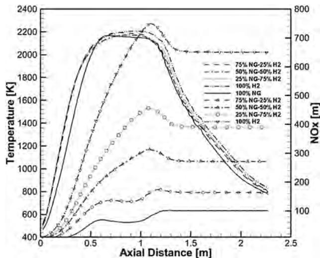
**Fig. 6 – The comparison of the natural gas and hydrogen-enriched natural gas axial temperature (shown with lines) and NO<sub>x</sub> gradients (shown with lines and symbols) distribution at the center line.**
