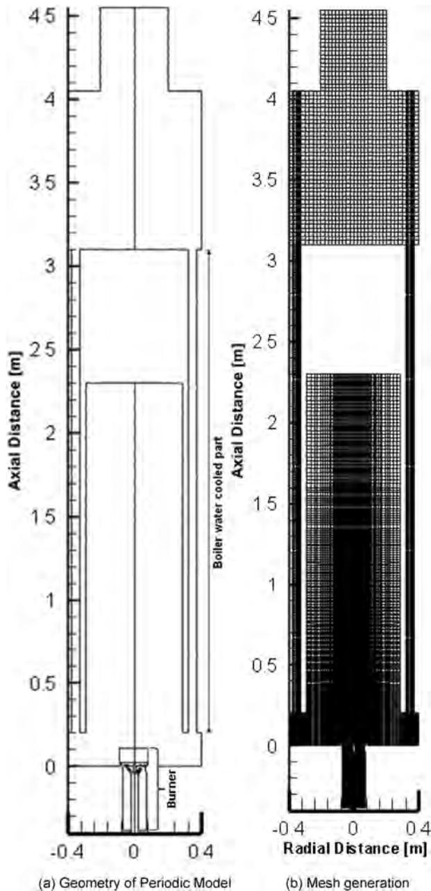
Fig. 3 – Periodic model (a) of the burner and boiler and mesh generation (b).
