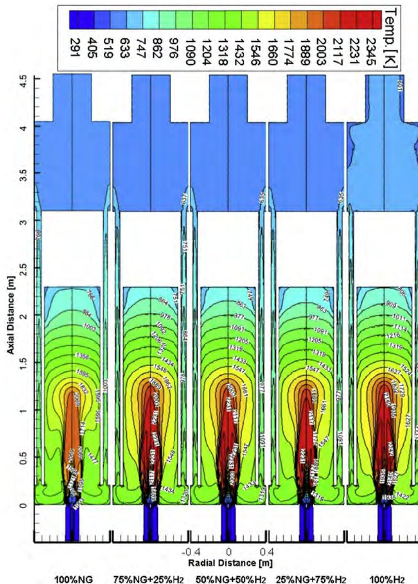
Fig. 5 – The effect of the hydrogen-enriched natural gas combustion on the temperature distribution.
