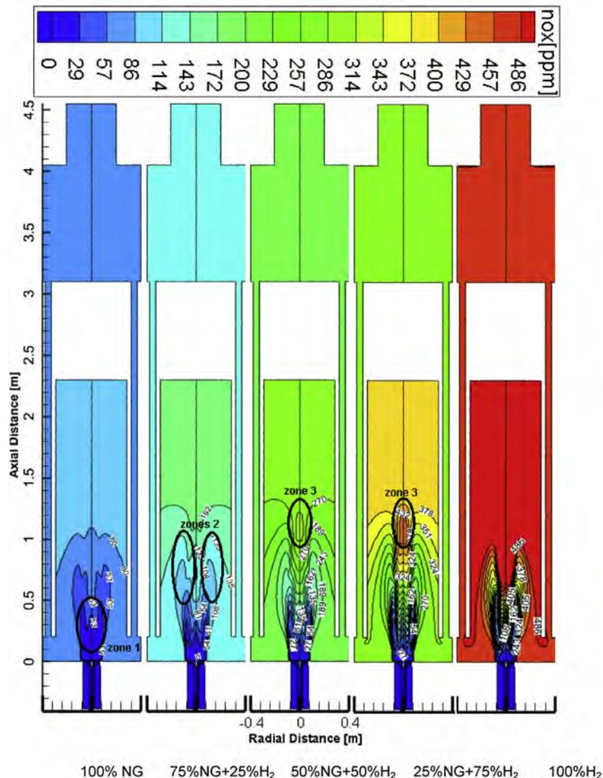
**Fig. 8 – The comparison of the NO<sub>x</sub> emissions of natural gas and hydrogen-enriched natural gas and hydrogen combustions at the yz plane.**
