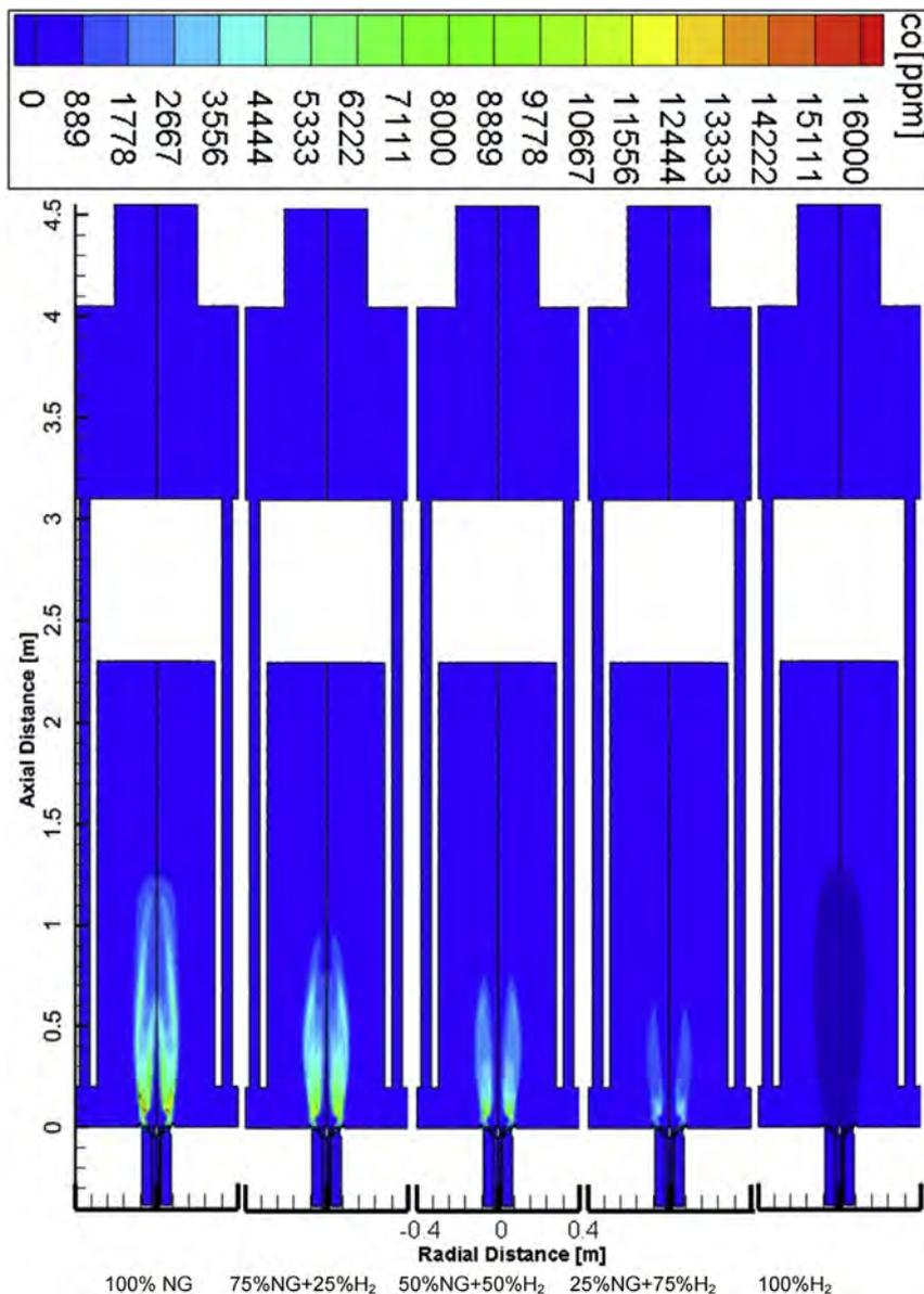
**Fig. 9** – The comparison of the CO emissions of natural gas, hydrogen-enriched natural gas and hydrogen combustions at yz plane.
