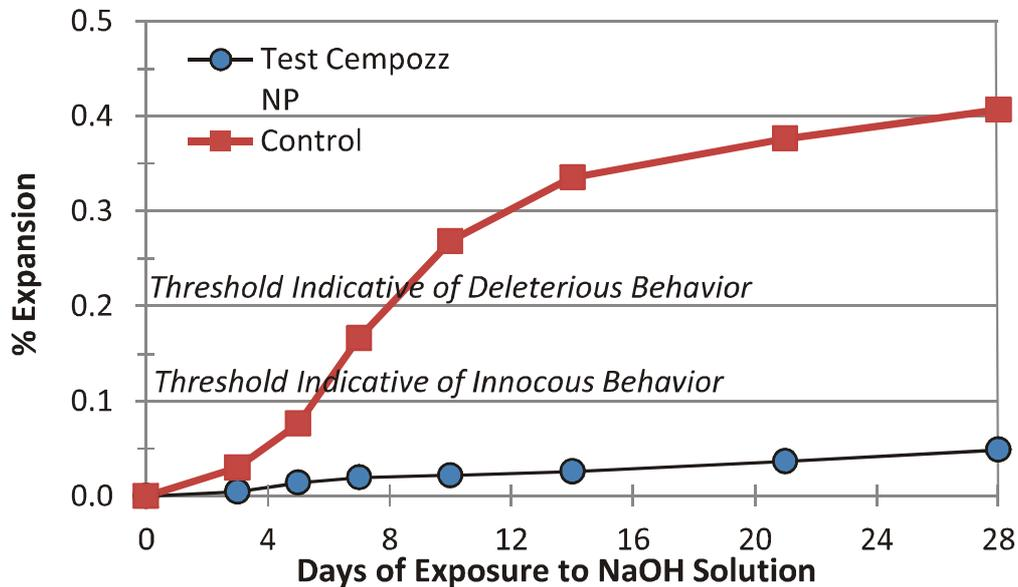
**Figure:** The Reduction in the Deleterious Expansion in Concrete Containing CemPozz®
